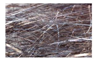
And this is what it looks like – uniquely formed metal fibres cool in production at 1 million degrees per second to create WoodMiser – measuring  $14 \text{ cm} \times 26 \text{ cm}$  (approx  $5.5^{"} \times 10^{"}$ ).
